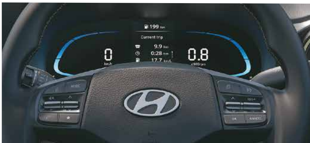
Advanced digital cluster with 10.67cm (4.2") coloured TFT MID and Tyre Pressure Monitoring System TPMS (Highline)
