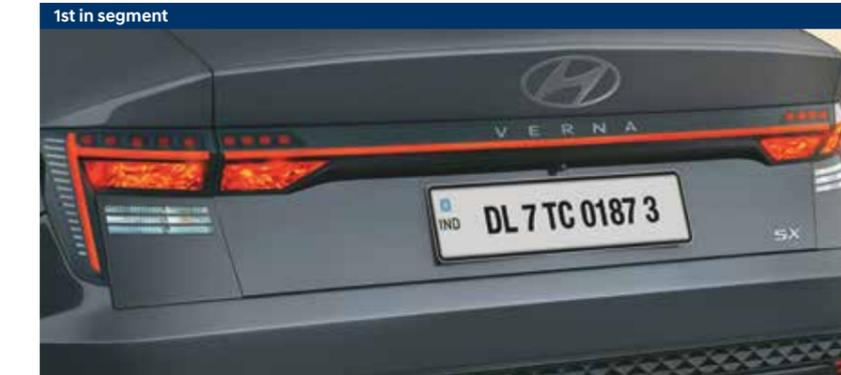
Parametric connected LED tail lamps
